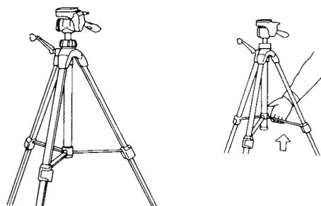
Holding two legs, one in each hand, tilt the tripod on its third leg. Pull the two legs you are holding outward, and all three legs will open at once. Open until the Center column ring is seated at the very bottom of the Center column.
