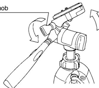
To rotate the camera left or right, loosen the Panning lock knob. When you want to lock in at a certain position, tighten the Knob.
