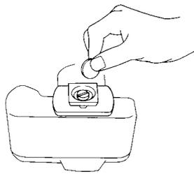
The retractable Camera positioning pin enables you to mount either a video, or a still camera on to the Quick release platform. For still cameras, align the length of the Platform along the baseplate of the camera body, and tighten screw into the tripod socket with a coin.
