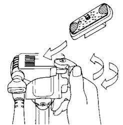
Return Quick release platform back onto the Pan head by inserting at an angle from the side closest to the Quick release lock lever.
