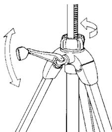
Loosen the Center column locking collar, and turn the Elevation crank handle to raise or lower the Center column.
