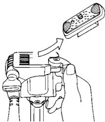
To remove the Quick release platform from the Pan head, turn Quick release lock lever counterclockwise, and lift Platform out at an angle from the side closest to the lever.
