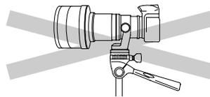
This product has been designed to handle equipment weighing under 2 kgs (4 lbs 6 oz). Do not overload. Some equipment weighing under 2 kgs (4 lbs 6 oz), such as long lenses, may not balance well due to its weight distribution. In such case, please use a larger tripod.
