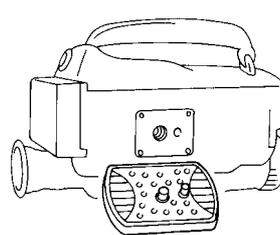
For video cameras, match the Camera positioning pin of the Platform to the corresponding hole beneath the camera, and then tighten screw into tripod socket with a coin. Replacement Quick release platform for the U 8000 is available. Cat. No. 618-731
