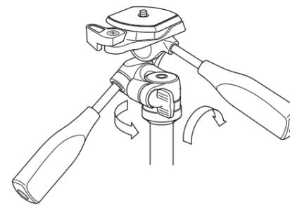
Use the following instructions if you wish to change heads, or attach accessories. First, lock the Panning Lock Knob, then grasp the Pan, or Vertical Tilt Handle and turn the head, counter-clockwise to loosen.
