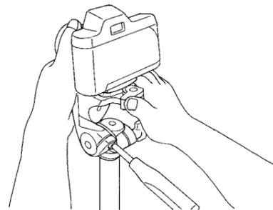
When attaching the camera to the Pan Head, check to make sure that the Quick Release Platform is engaged in the catch of the Pan Head before locking the lever.
