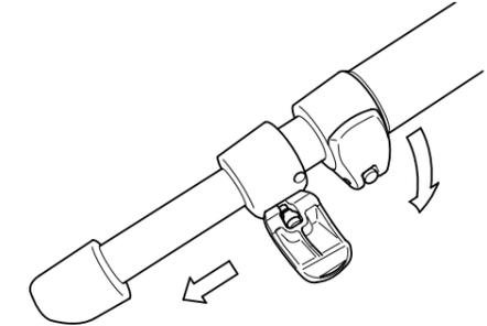
Open the Leg Lock Lever for extending/folding of tripod legs. Lock the lever tightly at your required position.
