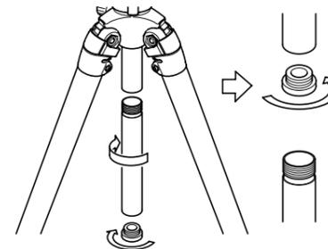
Remove the center column Base Stopper and then, remove the lower part of the center column. Put the center column Base Stopper on the upper part of the center column.
