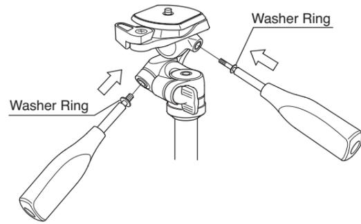
Attach the two Pan Handles to the Pan Head, by inserting the shorter handle to the left, and the longer handle to the right. Do not reverse.
