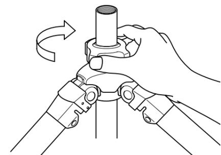
Insert the Center Column from the lower side of Main Body, and tighten the Locking Collar and the Center Column Stopper.
