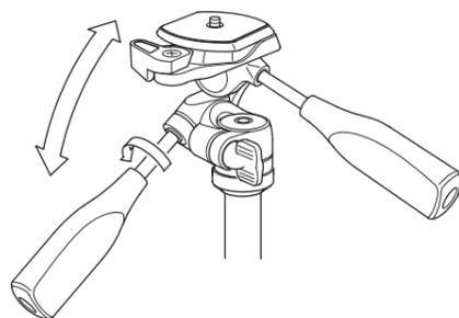
Loosen the Pan & Tilt Handle, and the head will tilt back and forth.
