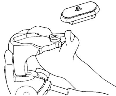
To remove the Quick Release Platform from the Pan Head, turn Quick Release Lock Lever and lift out Platform from its back.
