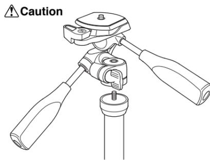
Remove the Pan Head when inverting &/or replacing the Center Column.
