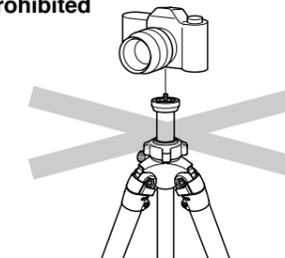
Do not attach camera directly to the threaded post of the Center Column. This may damage both camera and tripod.
