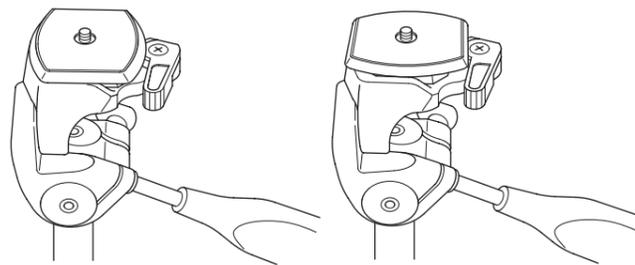
The Quick Release Platform can be attached to the camera body in either directions (along the length, or along the width). This feature facilitates your camera set up into the vertical position, simply by the turn of one of the tilt handles.
