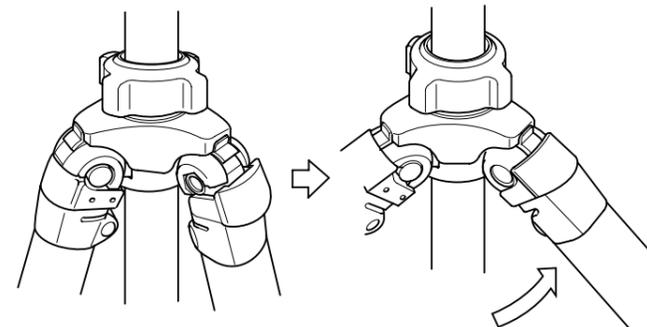
To change the angle of each leg, close the Leg slightly, and then pull the Leg Angle Adjustment Lock out. There is a choice of two other angle positions.
