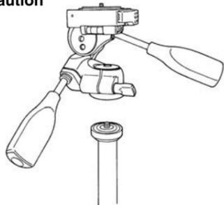
Always remove the Pan Head when replacing the Center Column.
