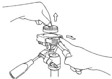
Remove Quick Shoe by opening the Locking Lever and then pressing the Release Button.
