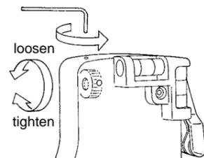
After long use, you may need to re-tighten the Lever Lock mechanism through the window located underneath the Pan Head. First, you will need to loosen the locking pin with an ordinary allen wrench(1.5 mm). We advise you not to tamper with this part until it becomes necessary.
