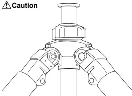
Make sure to re-attach the Center Column Base Stopper, in order to prevent the Center Column from falling out.
