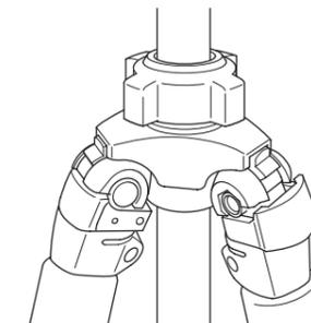
To change the angle of each leg, close the Leg Angle Adjustment Lock out. There is a choice of two other angle positions.
