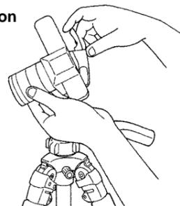
The camera may fall suddenly when the Locking Lever is loosened, causing damages and injuries. Always hold on to the camera during such operation.
