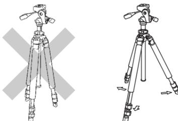
Be sure to open all three legs completely in order to prevent camera shaker, or accidental tip overs caused by unstableness.
