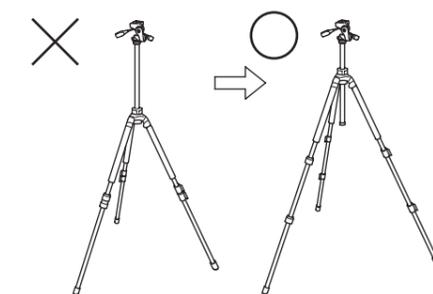
To avoid unnecessary camera vibrations, try to keep the Center Column height to a minimum. Also use the larger legs first, when extending the legs.
