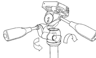
Please exchange by the following method to attach other heads or accessories to this leg. Fix the Center Column of the legs firmly by both the Center Column Locking Collar and the Center Column Stopper. Next, tighten the Panning Lock Knob of the head firmly. The Pan & Tilt Handle and the Vertical Tilt Handle are grasped and then, turn the head counter-clockwise forcibly. The head loosens now.
