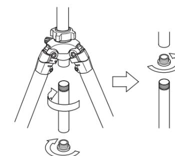
Remove the Center Column Base Stopper and then, remove the Lower part of Center Column. Put the Center Column Base Stopper on the Upper part of Center Column.
