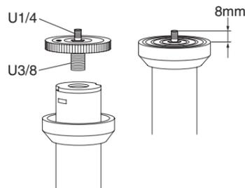
4. Loosen the Pan Head fixing screw and pull it out. Then, screw it in again after reversing top and bottom.
