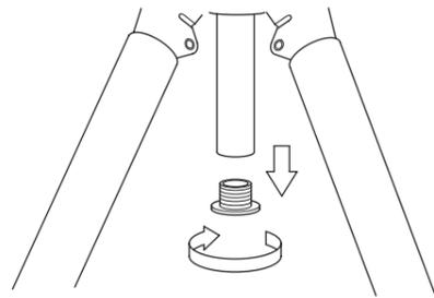
Remove the Center Column Base Stopper turning to the way of arrow.
