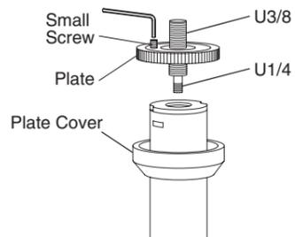
The Pan Head fixing screw is reversible for either large thread (U3/8) or small thread (U1/4).
