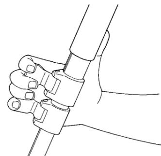
Flip up the Leg Lock Lever to extend or shorten any of the individual leg sections to the desired length, and press the Leg Lock Lever flush against the Leg to lock.
