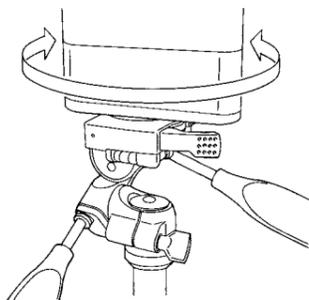
Correctly installed you will hear a "click", and the Quick Shoe will rotate 360°.
