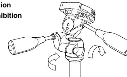
Set the new head, or accessory on the tripod's threaded post, and turn clockwise until it comes to a stop. Tighten the Panning Lock Knob and turn clockwise slightly more. Do not attach camera directly to the threaded post of the Center Column. This can damage both camera and tripod.
