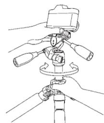
Hold onto the Pan Head with one hand, and loosen the Center Column Stopper and the Center Column Locking Collar with the other hand. Raise or lower Pan Head to desired height, and while maintaining a hold of the Pan Head, tighten the Locking Collar and the Stopper.
