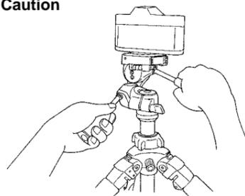
When loosening either the Pan & Tilt Handle, or the Vertical Tilt Handle, take precaution by keeping a firm grip on the handle until the Pan Head is locked down.
