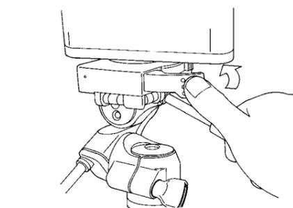
Fix the Quick Shoe at a desired position by closing the Locking Lever.
